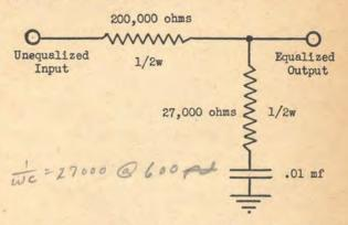
circuit shown, when substituted for the *Clarkstan* circuit, will give a response flat within 2 db. from 50 to 10,000 cycles (when tested with use of a sweep frequency record) and a voltage output at 1000 cycles of 7 millivolts.
