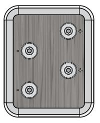
Loosen the terminals. Remove the straps Re-tighten all terminals hand tight
